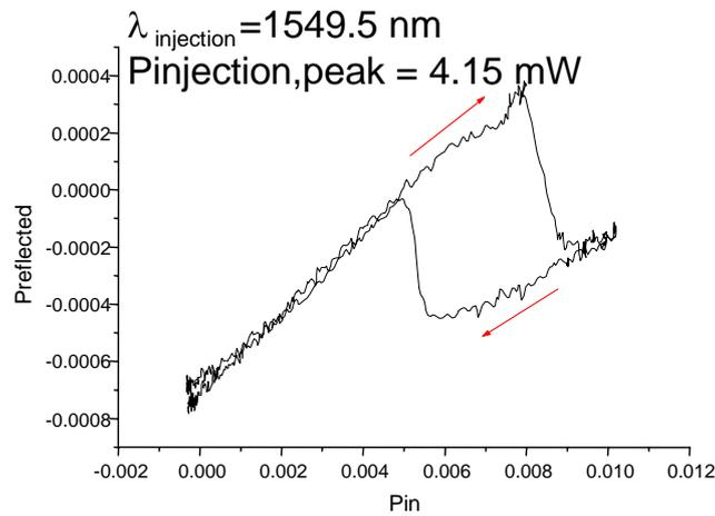
Figure 15: Optical bi-stability effect in a 2.5D PC structure as shown in figure 13
