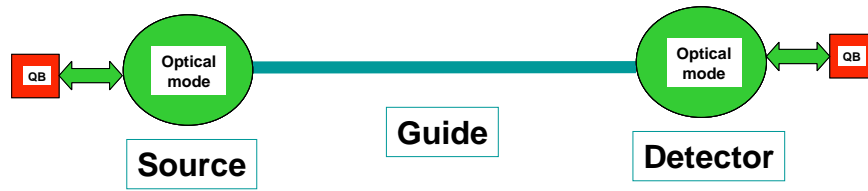
Figure 9: schematic view of a quantum optical link
