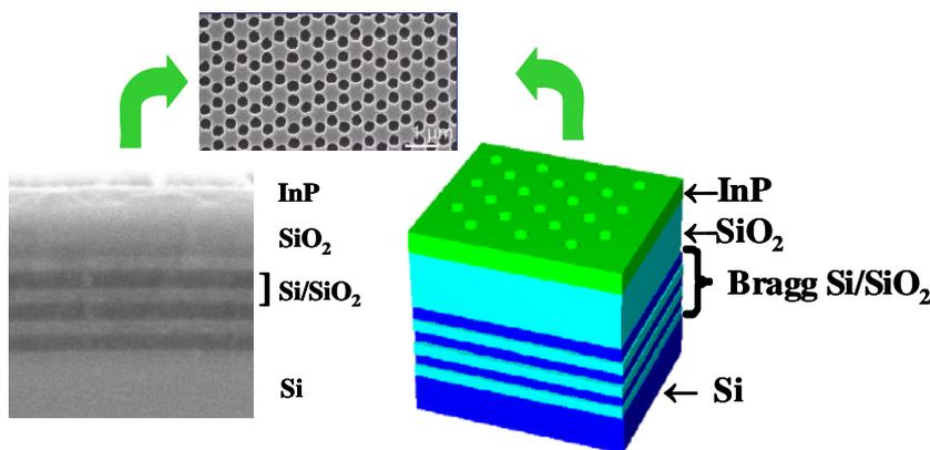
Figure 13: Photonic Crystal membrane bonded on top of a Bragg
