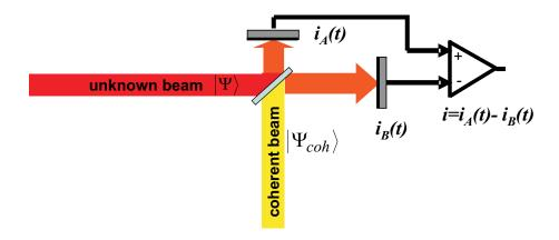
Figure 2: Balance homodyne detection set-up
