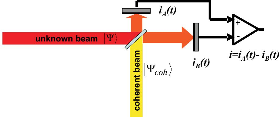
Figure 2: Balance homodyne detection set-up
